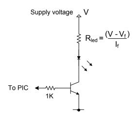
V is the power supply voltage  $R_{\text{led}}$  is the current limit resistor value
